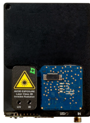
Combined optical assembly with spectrometer and two temperature-controlled lasers
