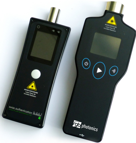
Hand-held optical test devices including light sources and spectrometer
